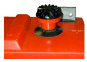
HYDROCAPS ARE ABLE TO CATALYTICALLY RECOMBINE THE HYDROGEN AND OXYGEN GASSES INTO PURE WATER WHICH RETURNS TO THE BATTERY CELL. THIS DRASTICALLY REDUCES THE AMOUNT OF "TOPPING UP" AND VIRTUALLY ELIMINATES THE DANGER OF A HYDROGEN GAS EXPLOSION. CORROSION IS ELIMINATED BECAUSE THE ACID SPRAY AND FUMES ARE CONTAINED WITHIN THE CELL.
